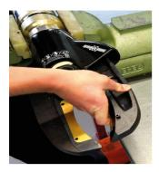
Next, the cutter is rotated and the blade insert is placed in the cutter blade with no insert. When inserting, make sure that the blade insert does not twist. If the blade inserts cannot be inserted by hand, use the
