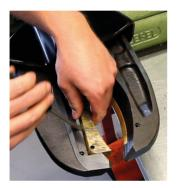
The cutter is positioned with the type plate pointing upward and is fixed in place. A clamping device, as shown in the illustrations, is not obligatory. When the blade insert is being changed, the battery must be removed from the cutter and not under load. This means that the shear is not completely open or closed. The blade insert for the cutter blade with the smooth surface can now be replaced. The roll pins are knocked out and downward from the punch (see figure 1).
