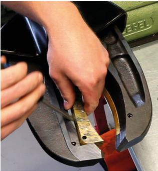
The cutter is positioned with the type plate pointing upward and is fixed in place. A clamping device, as shown in the illustrations, is not obligatory. When the blade insert is being changed, the battery must be removed from the cutter and not under load. This means that the shear is not completely open or closed. The blade insert for the cutter blade with the smooth surface can now be replaced. The roll pins are knocked out and downward from the punch (see figure 1).
