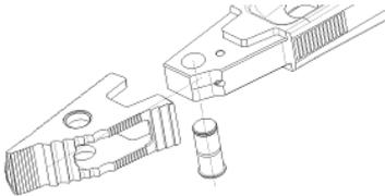
The collar studs on the spreader tips can be pressed out of the spreader arms but have a safety system to prevent them being lost and so they cannot be separated from the tips.
