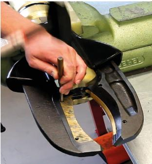
After the roll pins have been knocked out of their position, the blade insert can be pulled out. The use of a forked screwdriver is recommended. If the blade insert cannot be loosened immediately, it can be gently levered out using a punch in the holes (see figure 2).
