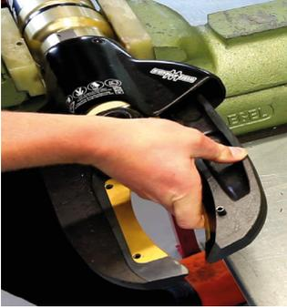
Next, the cutter is rotated and the blade insert is placed in the cutter blade with no insert. When inserting, make sure that the blade insert does not twist. If the blade inserts cannot be inserted by hand, use the soft-head hammer (see figure 3).
