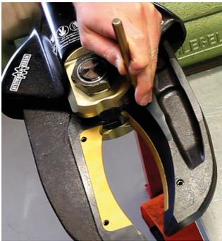
The roll pins are located using a punch and light blows of a hammer from above into the position holes provided for this purpose. Roll pins should be pushed into position until they are flush with the top surface of the blade (see figure 4).
